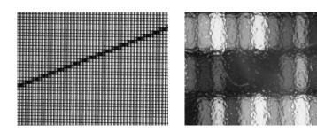
The left image is magnified 20x; the right image 400x. The rectangular shapes you can see in the images are the separate Red, Green, and Blue sub-pixels, which a monitor uses to build up all the different colours and greys it may need (the monitor makes a picture by emitting light and Red, Green, and Blue are the primary colours of light.)
